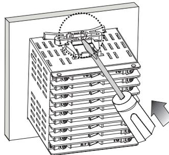
※Mount the unit on the panel. Push the bracket with tools to fix the unit as the figure.
