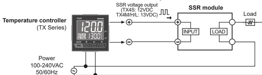
※When selecting cycle or phase control mode, the power supply for a load and a temperature controller must be the same.
