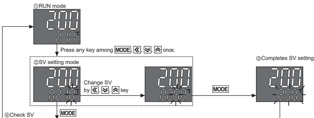
※If there is no key input for 3 sec while setting SV, the new setting is applied and the unit will return to RUN mode.
