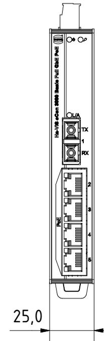
for mounting rail acc.to DIN EN 60715
