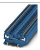
Disconnect terminal block, Connection type: Push-in connection, Cross section: 0.14 mm² - 1.5 mm², AWG: 26 - 14, Nominal current: 10 A, Nominal voltage: 400 V, Length: 58.9 mm, Width: 3.5 mm, Color: blue, Assembly: NS 35/7,5, NS 35/15
