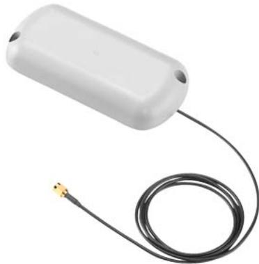
ANT794-3M mobile wireless antenna for 2G, GSM networks, flat antenna for 900/1800/ 1900 MHz; weatherproof for indoor and outer area; 1.2 m Connection cable permanently connected to the antenna; SMA connector; incl. adhesive tape for mounting.
