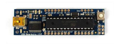
Next, you can attach header pins to make the USB Boarduino fit nicely into a breadboard. If you want to solder wires to the pins instead (free-wiring) you should skip this step.
