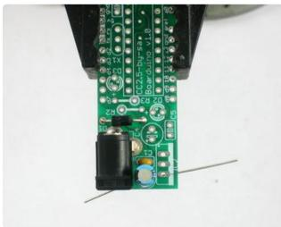
Next, its time to place the 25V electrolytic capacitor C3. Electrolytic capacitors are polarized which means they only work well in one direction. Put it in backwards and they can explode! You can tell how to place it because the silkscreened image has a plus near one hole and the capacitor has one long lead. That lead is the positive lead. In this image, its the one on the right.
