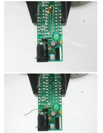
The 1K resistor R2 goes in, its the LED's matching resistor. Bend it over as shown to place it.
