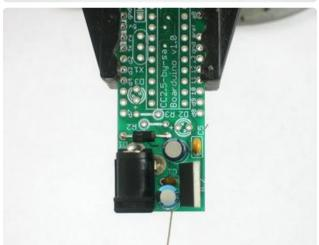
Now you should soder in the 6.3V electrolytic capacitor C4 as shown. Remember its polarized so you must place the longer lead in the positive-marked hole.
