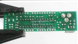
Solder in the socket by tacking two opposite corners and then soldering the rest of the pins. Press the socket into the board to make sure its flat up against it.
