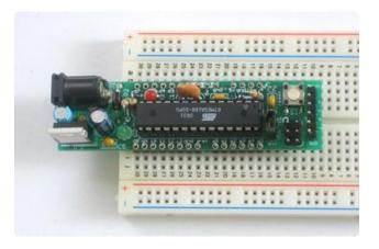
Place the Boarduino on top, so that the header matches up with the solder holes in the PCB.
