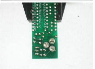
Solder in the resistor and LED and clip the leads.
