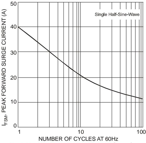
Fig. 5 Max Non-Repetitive Peak Forward Surge Current
