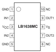
Note: both ground pins must be grounded.
