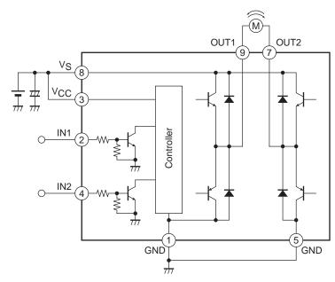
Note: When using the same power supply for  $V_S$  and  $V_{CC}$ , short the  $V_{CC}$  and  $V_S$  pins to each other or insert a capacitor in the  $V_{CC}$  line.
