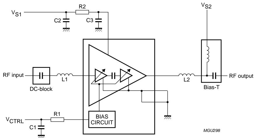
Fig.10 Test diagram.
