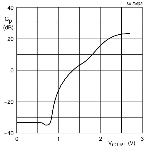
$V_S = 3 \text{ V}; P_D = -14 \text{ dBm}; f = 1.9 \text{ GHz}$ .
