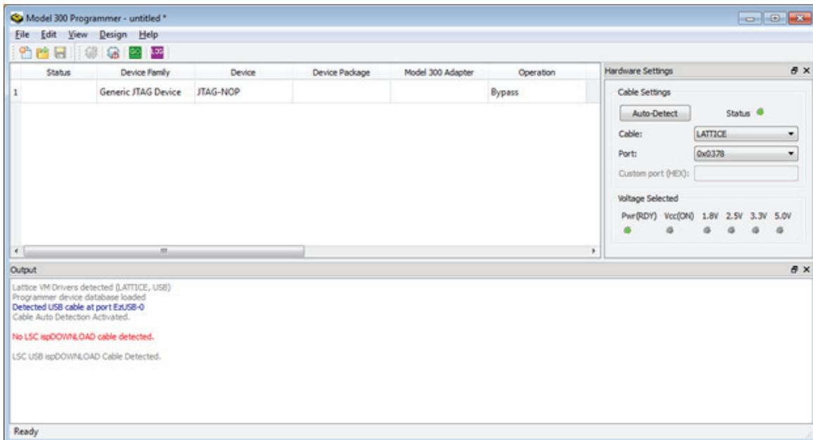
Edit **Device Family**, **Device** and **Device Package** to select the appropriate settings. Verify the “Model 300 Adapter” setting. Double click the Operation field to select the desired operation and Programming file:
