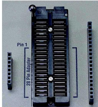
2. Using proper ESD handling procedures, place the device in the programming adapter socket, and ensure the correct alignment of the device.
