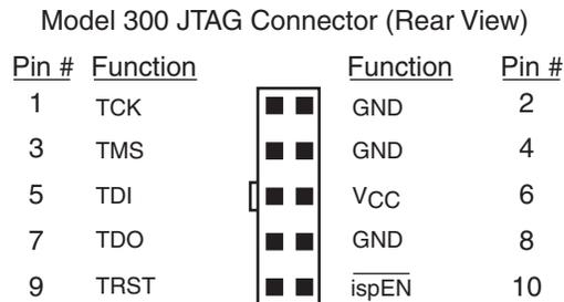
When connecting to the Model 300 programmer JTAG connector, eight wires must be connected from the programming cable: TCK, TMS, TDI, TDO, TRST, ispEN, Vcc and GND. It is sufficient to connect the programming cable GND wire to a single JTAG connector GND pin: 2, 4 or 8. See UG48, [ispDOWNLOAD Cables User's Guide](#) for the full specifications of the cable and 10-pin connector.
