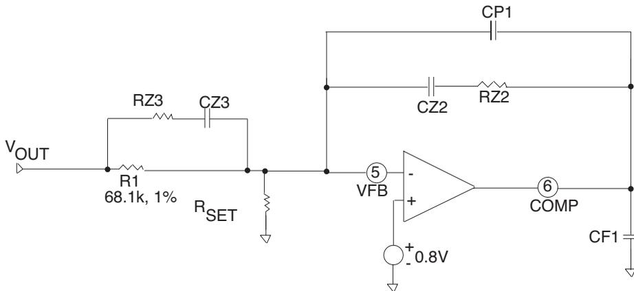
$$R_{SET} = 54.48 / (V_{OUT} - 0.8) \text{ (k}\Omega\text{)}$$
