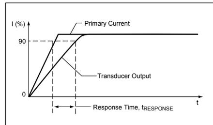
**Rise time ( $t_r$ ).** The time interval between a) when the sensor reaches 10% of its full scale value, and b) when it reaches 90% of its full scale value. The rise time to a step response is used to derive the bandwidth of the current sensor, in which  $f(-3\text{ dB}) = 0.35/t_r$ . Both  $t_r$  and  $t_{RESPONSE}$  are detrimentally affected by eddy current losses observed in the conductive IC ground plane.
