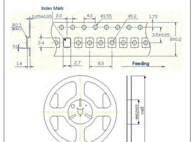
1. 230mm minimum leafer which consist of carrier and/or tape followed by a minimum of 160mm of empty carrier tape sealed with cover tape.
