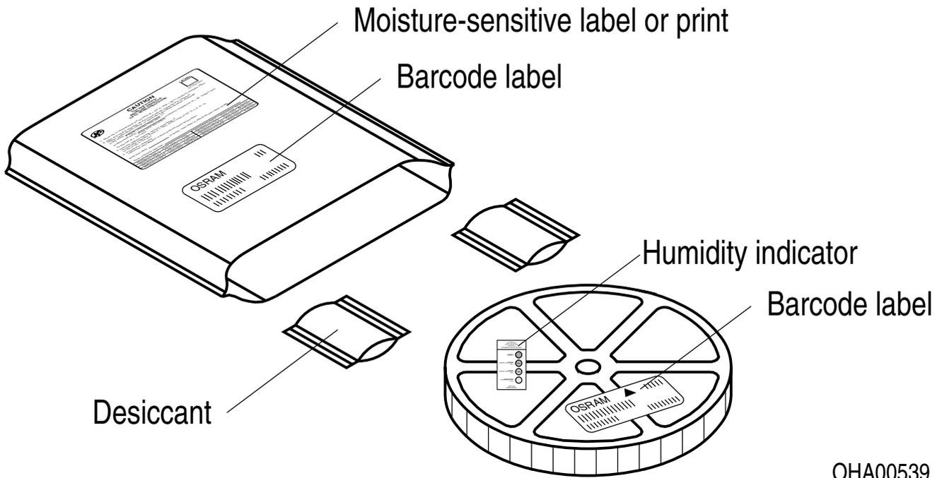
Moisture-sensitive product is packed in a dry bag containing desiccant and a humidity card according JEDEC-STD-033.
