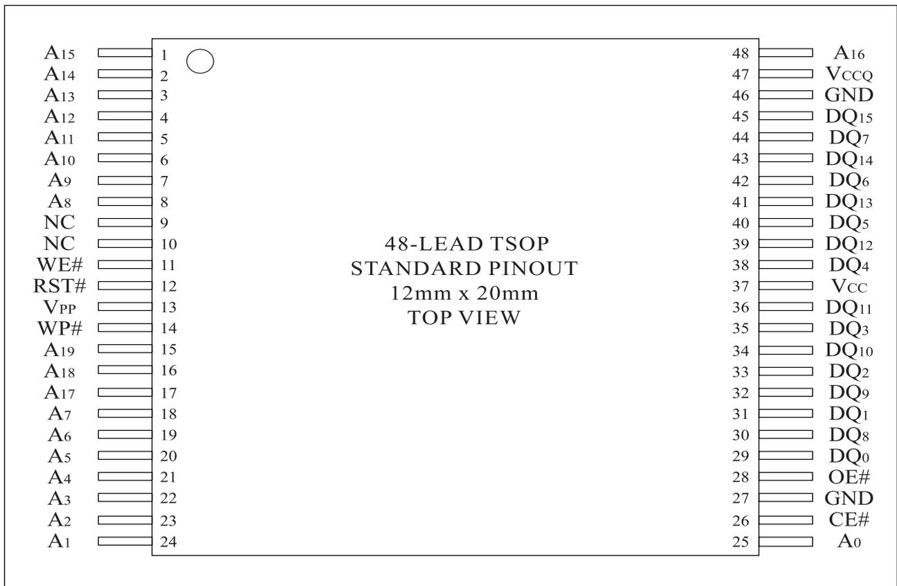
Figure 1. 48-Lead TSOP (Normal Bend) Pinout
