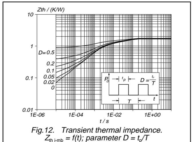
Silicon Diffused Power Transistor
