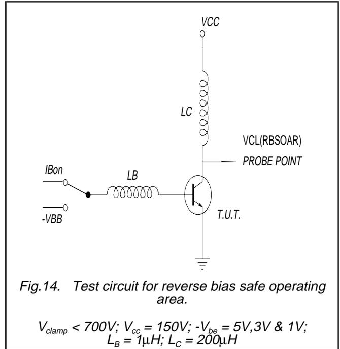
Fig.14. Test circuit for reverse bias safe operating area.
