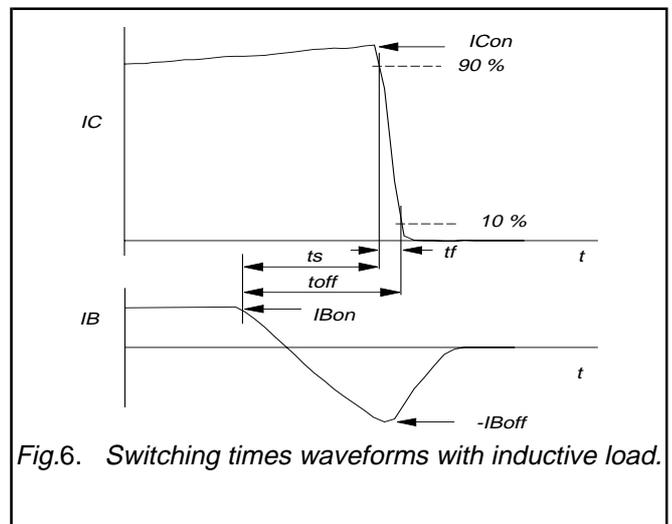
Silicon Diffused Power Transistor
