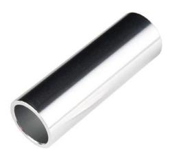
**Description:** These 2" long aluminum tubes have an outer diameter of 1", an inner diameter of 0.82", and a wall thickness of 0.09". When used with the mating tube clamps, these can be used for versatile structural support. Additionally, wires and cables can easily be run through the center.
