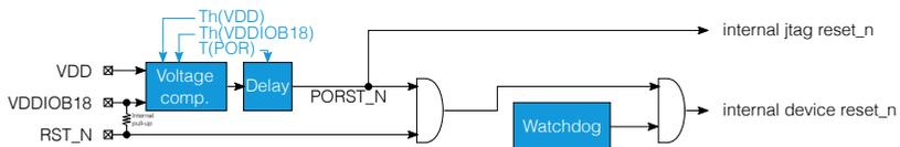
When the device comes out of reset, the boot procedure starts (Section 9). The chip can be reset externally using the RST\_N pin. If required, the JTAG state machine can be reset to its idle state by clocking TCK five times whilst TMS is high.
