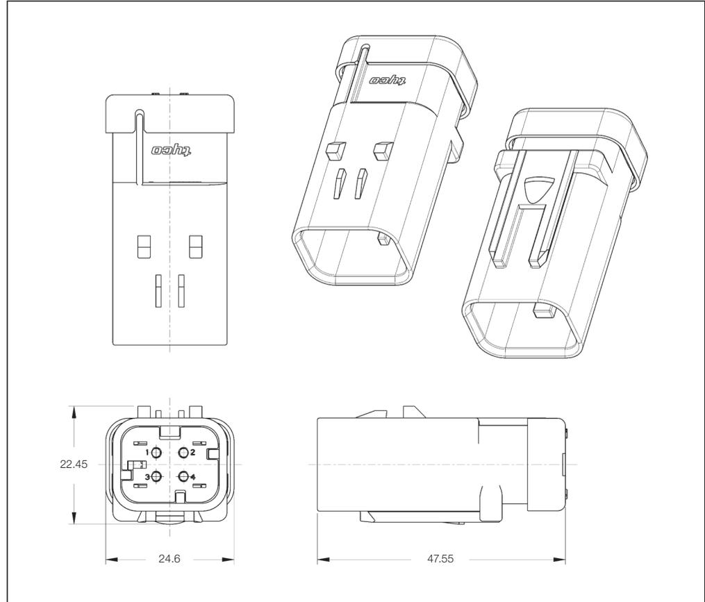
**Sealed Pin Housings 2-Row with Standard Diameter Wire Seal**
