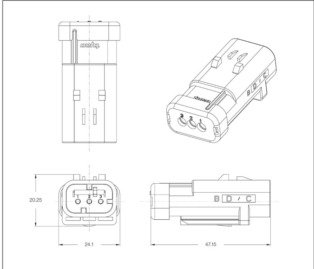
**Sealed Pin Housings 1-Row – Reversed Mounting Feature**
