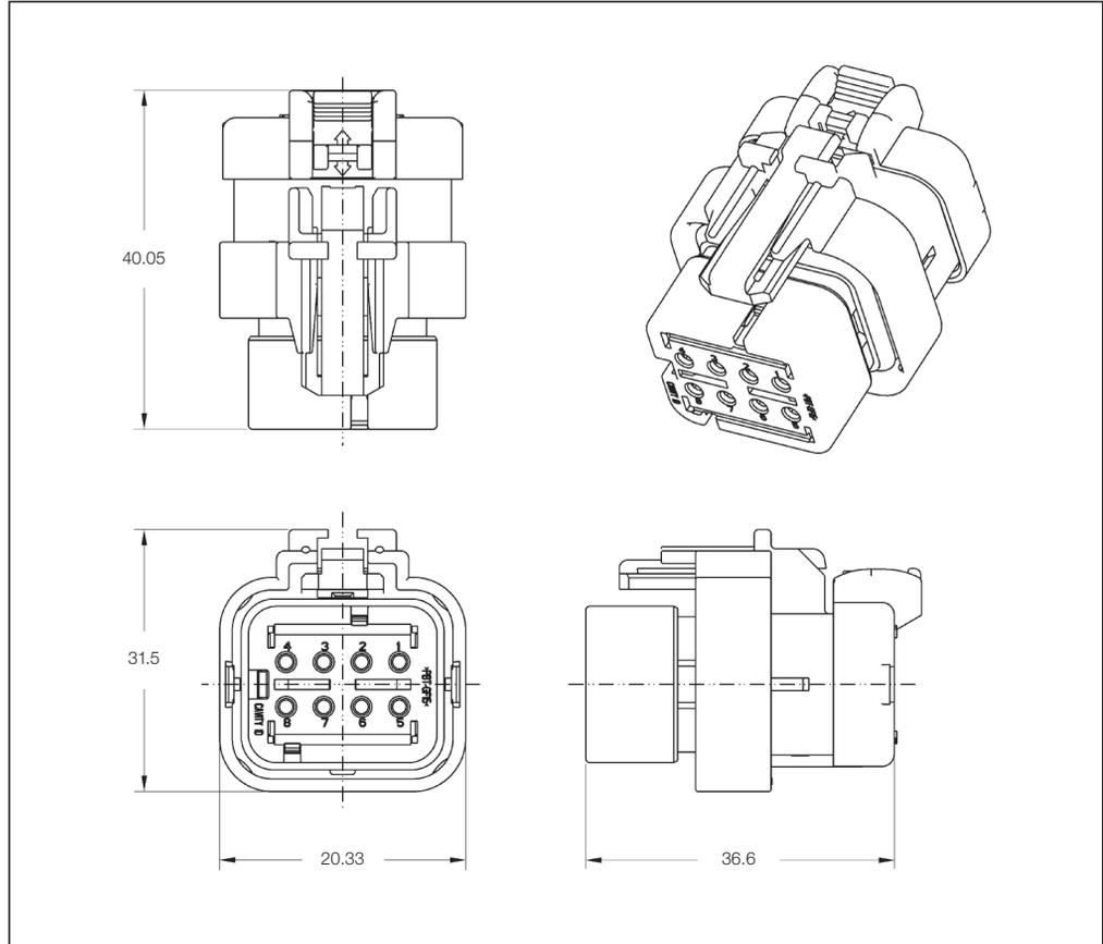
**Sealed Receptacle Housings 2-Row with Standard Diameter Wire Seal**
