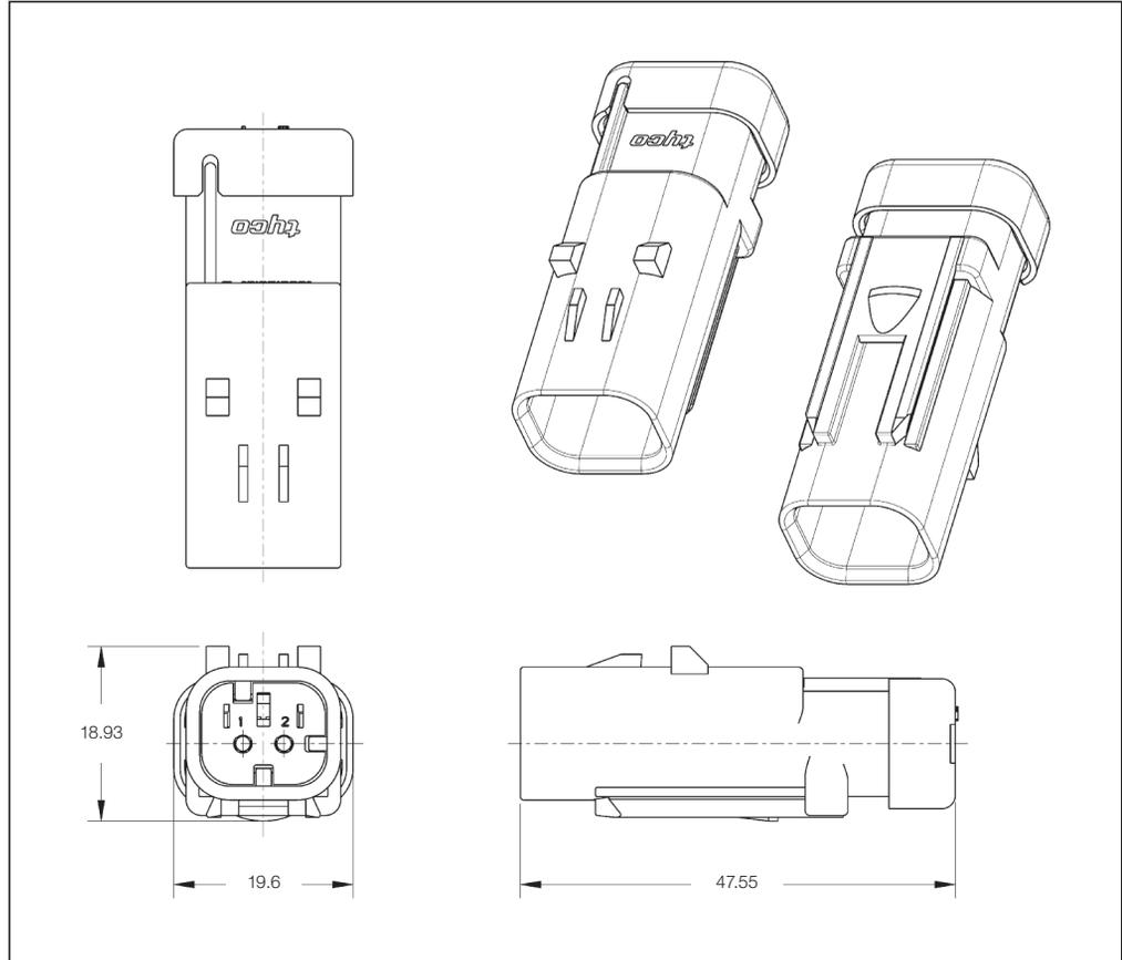
**Sealed Pin Housings 1-Row with Standard Diameter Wire Seal**
