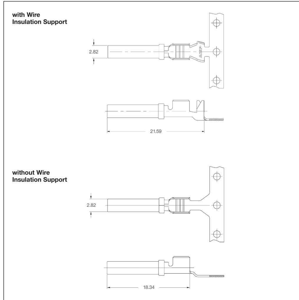
**Receptacle Contacts with Wire Insulation Support**
