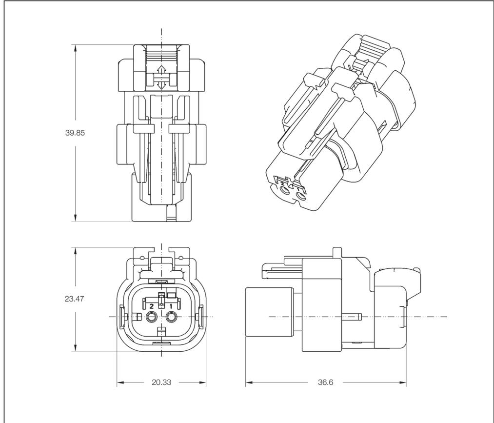
**Sealed Receptacle Housings 1-Row with Standard Diameter Wire Seal**
