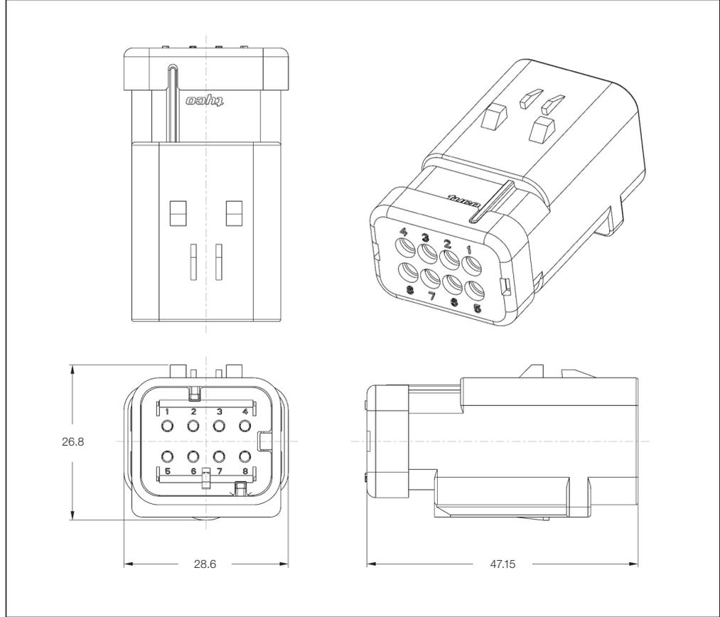
**Sealed Pin Housings 2-Row – Reversed Mounting Feature**
