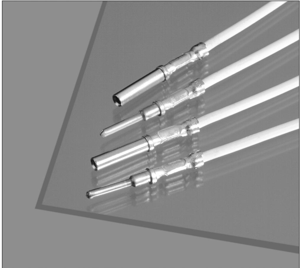
The HDSF Size 16 Pin and Socket contacts system is a stamped and formed version of the screw machine MIL-C-39029 contacts.
