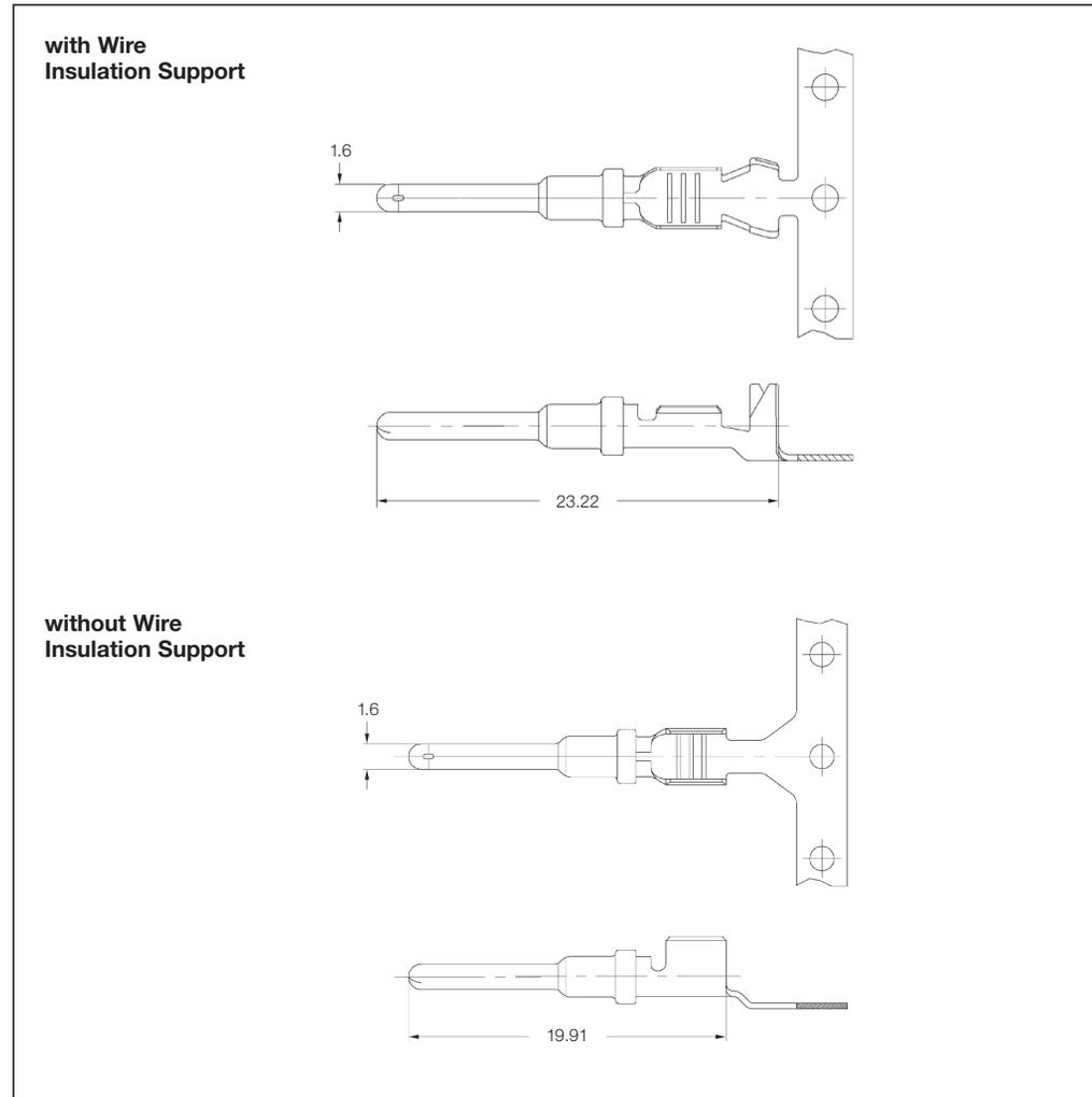
**Pin Contacts with Wire Insulation Support**
