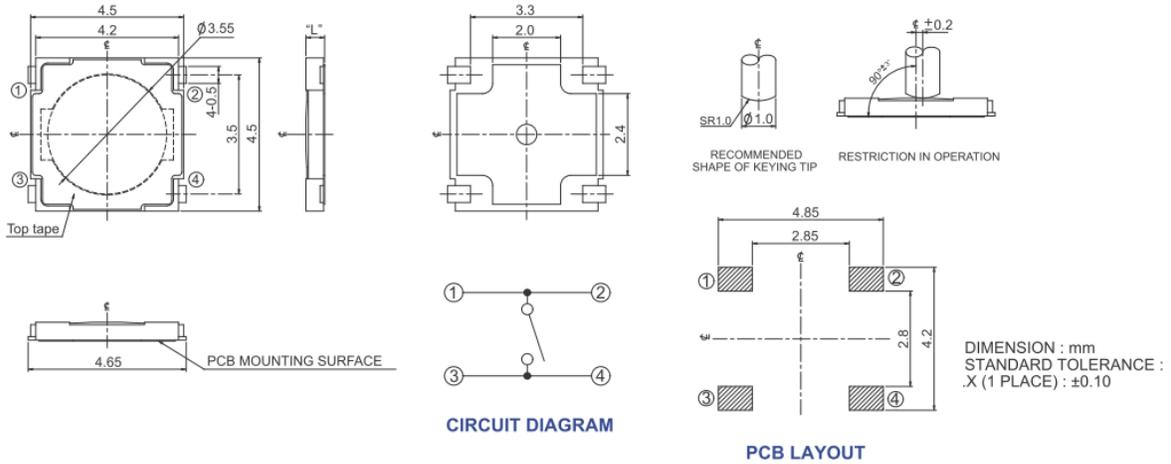
Figure 2 – 223BM2VA..., Surface Mount Gull Wing Type 2, Flat surface
