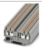
Feed-through terminal block, Connection method: Push-in connection, Cross section: 0.14 mm<sup>2</sup> - 4 mm<sup>2</sup>, AWG: 26 - 12, Width: 5.2 mm, Height: 35.3 mm, Color: yellow, Mounting type: NS 35/7,5, NS 35/15
