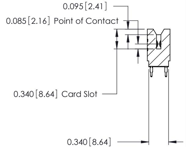
746 Series Ultra-Mate Card Edge Connector - Press Fit
