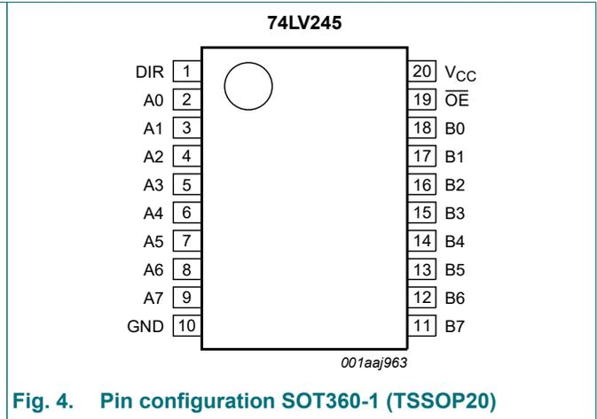
Fig. 4. Pin configuration SOT360-1 (TSSOP20)
