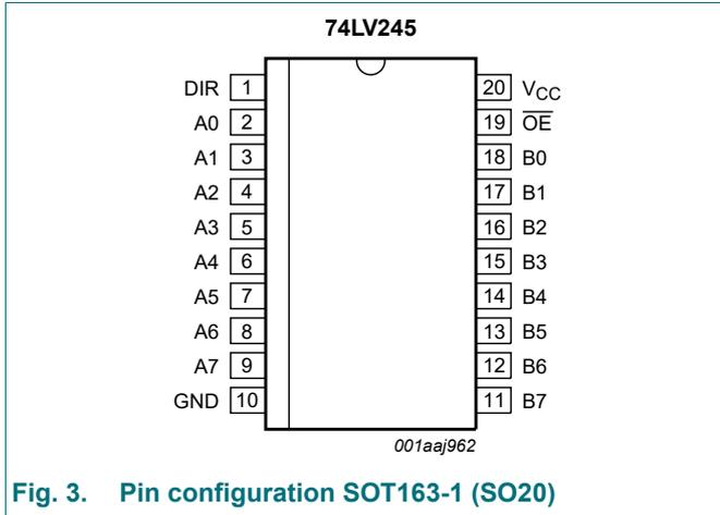
Fig. 3. Pin configuration SOT163-1 (SO20)
