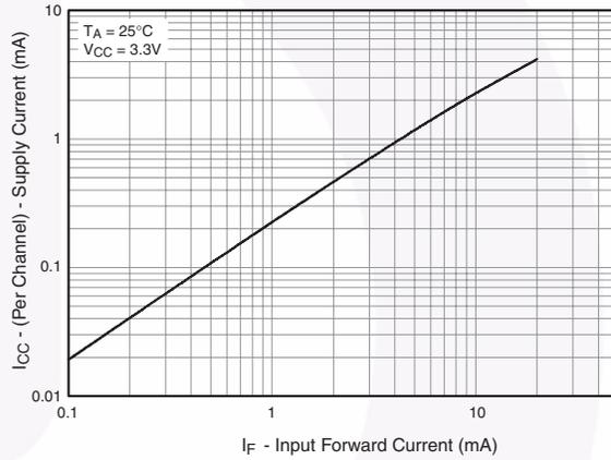
**Fig. 5 Output Current vs Input Forward Current**
