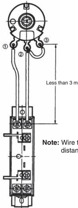
**Note:** Wire the external adjuster at a distance of less than 3 m.
