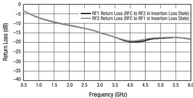
Figure 6. Return Loss vs Frequency (Isolation State)
