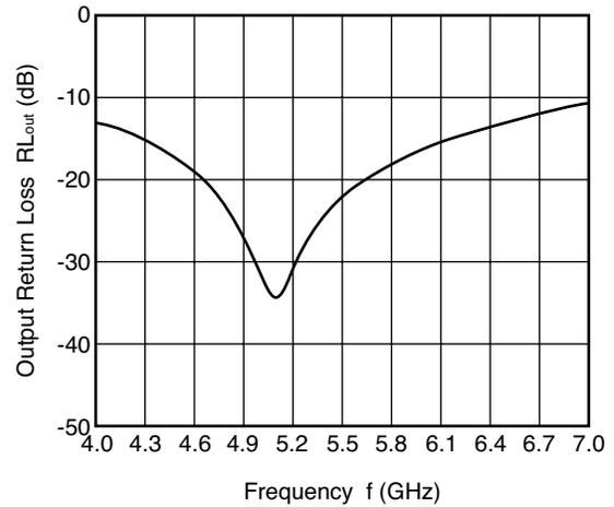
TX-ANT2 INPUT RETURN LOSS vs. FREQUENCY
