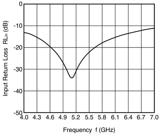
TX-ANT1 OUTPUT RETURN LOSS vs. FREQUENCY
