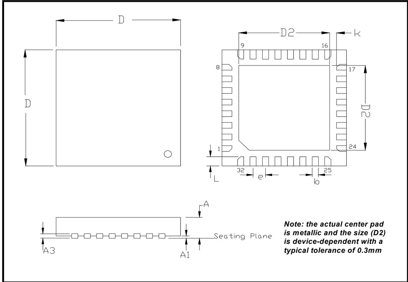
Note: The control dimension is in millimeter.
