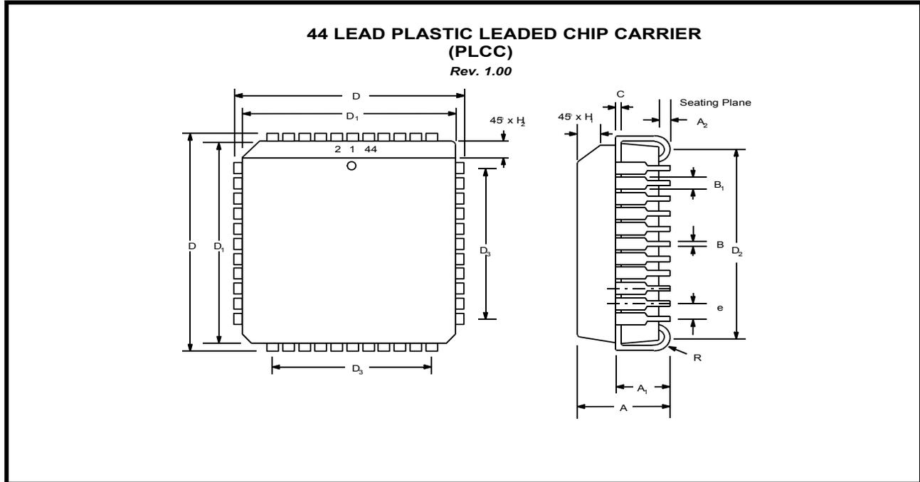
Note: The control dimension is the millimeter column
