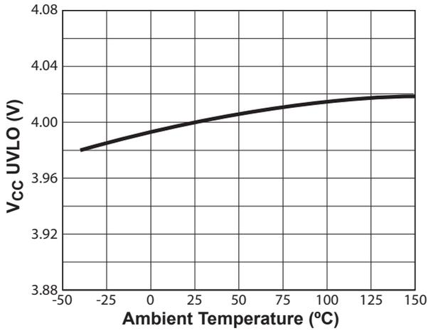
Figure 7.1 : V<sub>CC</sub> UVLO vs. Temperature
