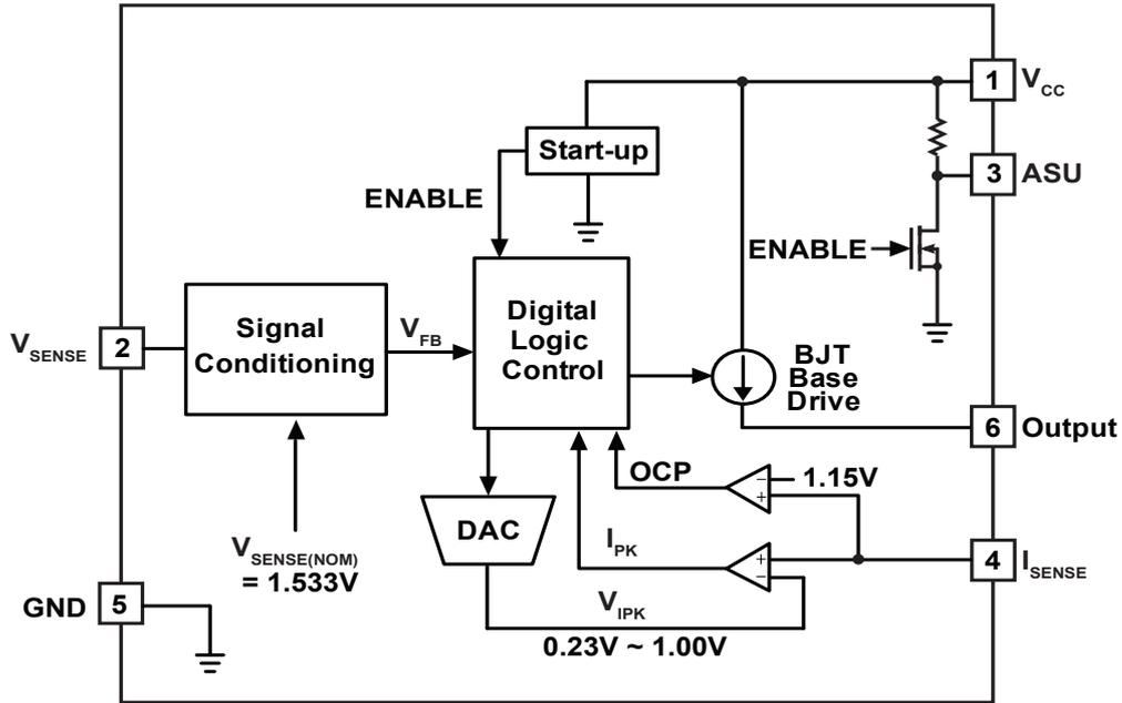
Figure 8.1 : iW1707 Functional Block Diagram
