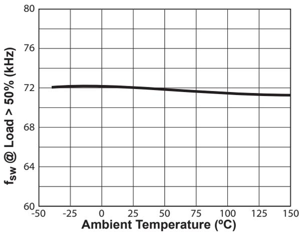
Figure 7.3 : Switching Frequency vs. Temperature<sup>1</sup>
