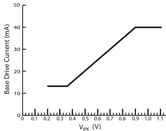
Figure 9.5 : Base Drive Current vs.  $V_{IPK}$
