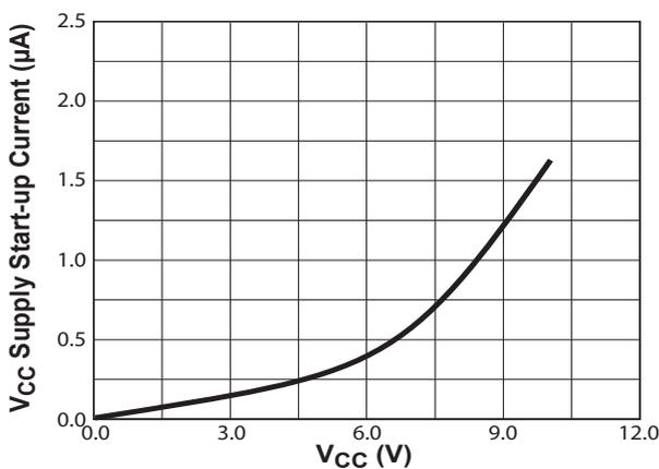
Figure 7.5 : V<sub>CC</sub> vs. V<sub>CC</sub> Supply Start-up Current
