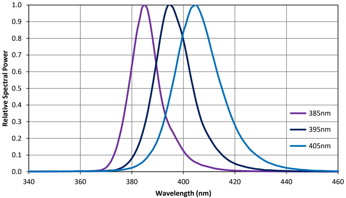
Figure 5: Relative spectral power vs. wavelength @  $T_c = 25^\circ\text{C}$ .
