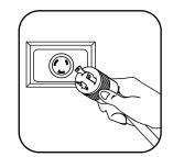
AC Input Connection: Insert L5-20P twist-lock plug into compatible L5-20R utility, generator or UPS outlet. (Included adapter converts L5-20P to 5-20P.)
