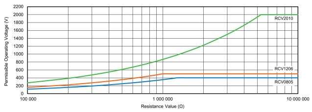
The permissible operating voltage  $U_{\rm max.}$  equals the rated voltage. For ambient temperatures above 70 °C power derating must be considered
