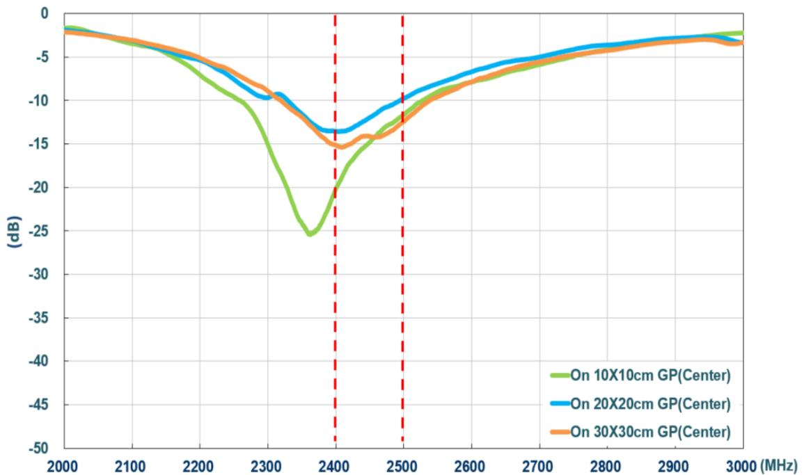
**Figure 3.** Return loss of WCM.01 on center of different ground plane sizes
