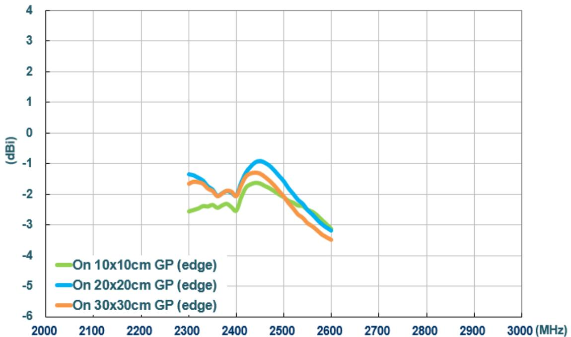
**Figure 13.** Average gain of WCM.01 on edge of different ground plane sizes
