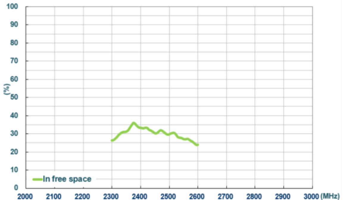
**Figure 5.** Efficiency of WCM.01 antenna in free space
