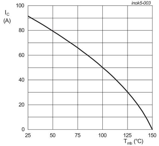
Fig. 3. Collector current as a function of case temperature
