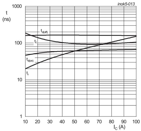
$R_g = 10 \Omega; V_{GE} = 15\text{V}/0\text{V}; T_j = 150 \text{ }^\circ\text{C};$
