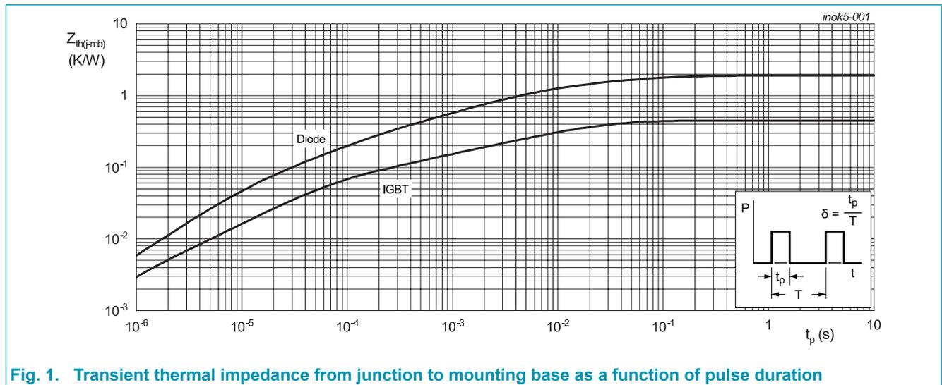
Fig. 1. Transient thermal impedance from junction to mounting base as a function of pulse duration
