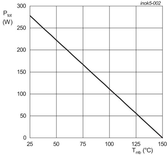
Fig. 2. Power dissipation as a function of case temperature
