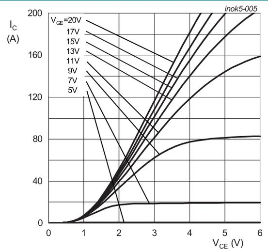
Fig. 5. Typical output characteristic
