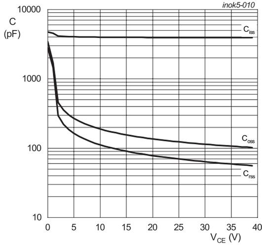
$V_{GE} = 0 \text{ V}; f = 1 \text{ MHz}$
