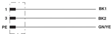
Contact assignment of the M12 plug
