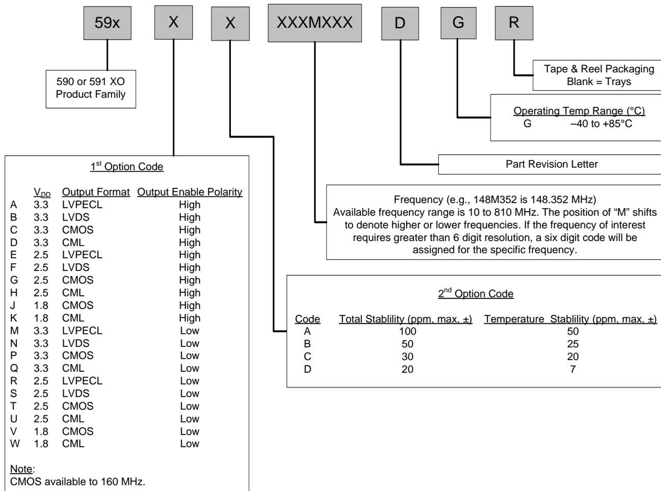
Example P/N: 590BB148M352DGR is a 5 x 7 XO in a 6 pad package. The frequency is 148.352 MHz, with a 3.3 V supply, LVDS output, and Output Enable active high polarity. Overall stability is specified as  $\pm 50$  ppm. The device is specified for  $-40$  to  $+85$  °C ambient temperature range operation and is shipped in tape and reel format.
