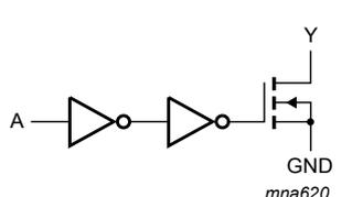
**Fig. 3. Logic diagram (one driver)**
