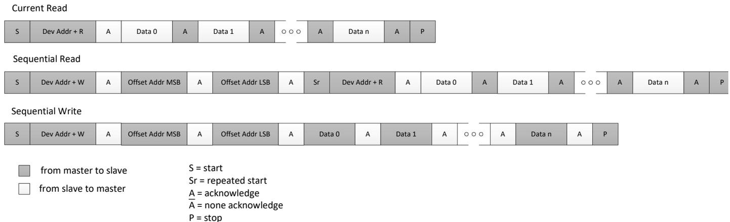
Figure 3. I<sup>2</sup>C Slave Read and Write Cycle Sequencing
