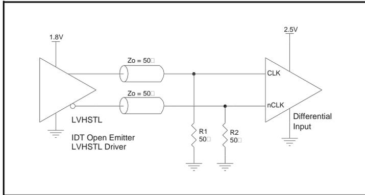
**Figure 8A.** CLKx/nCLKx Input Driven by an IDT Open Emitter LVHSTL Driver
