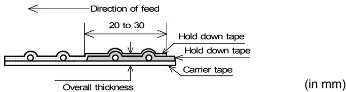
3. Both carrier tape and hold down tape
