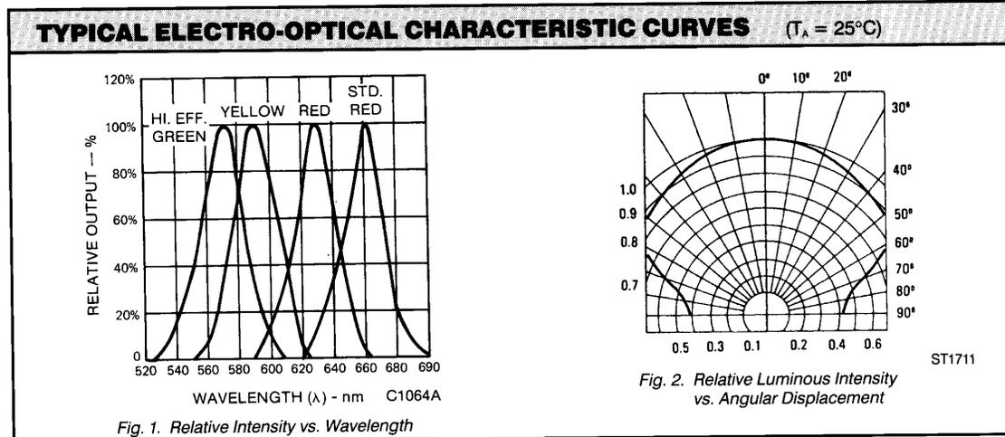
**TYPICAL ELECTRO-OPTICAL CHARACTERISTIC CURVES** ( $T_A = 25^\circ\text{C}$ )
