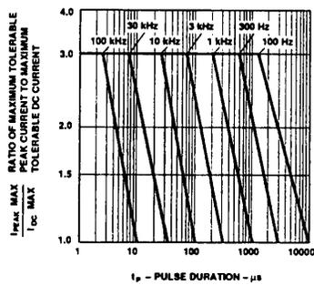
Fig. 5. Maximum Peak Current vs. Pulse Duration
