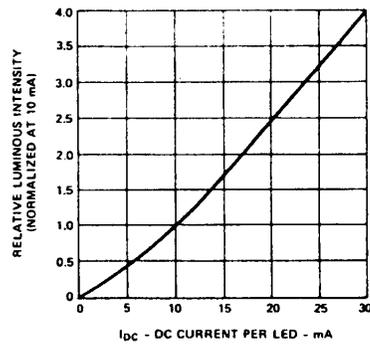
Fig. 4. Relative Luminous Intensity vs. DC Forward Current
