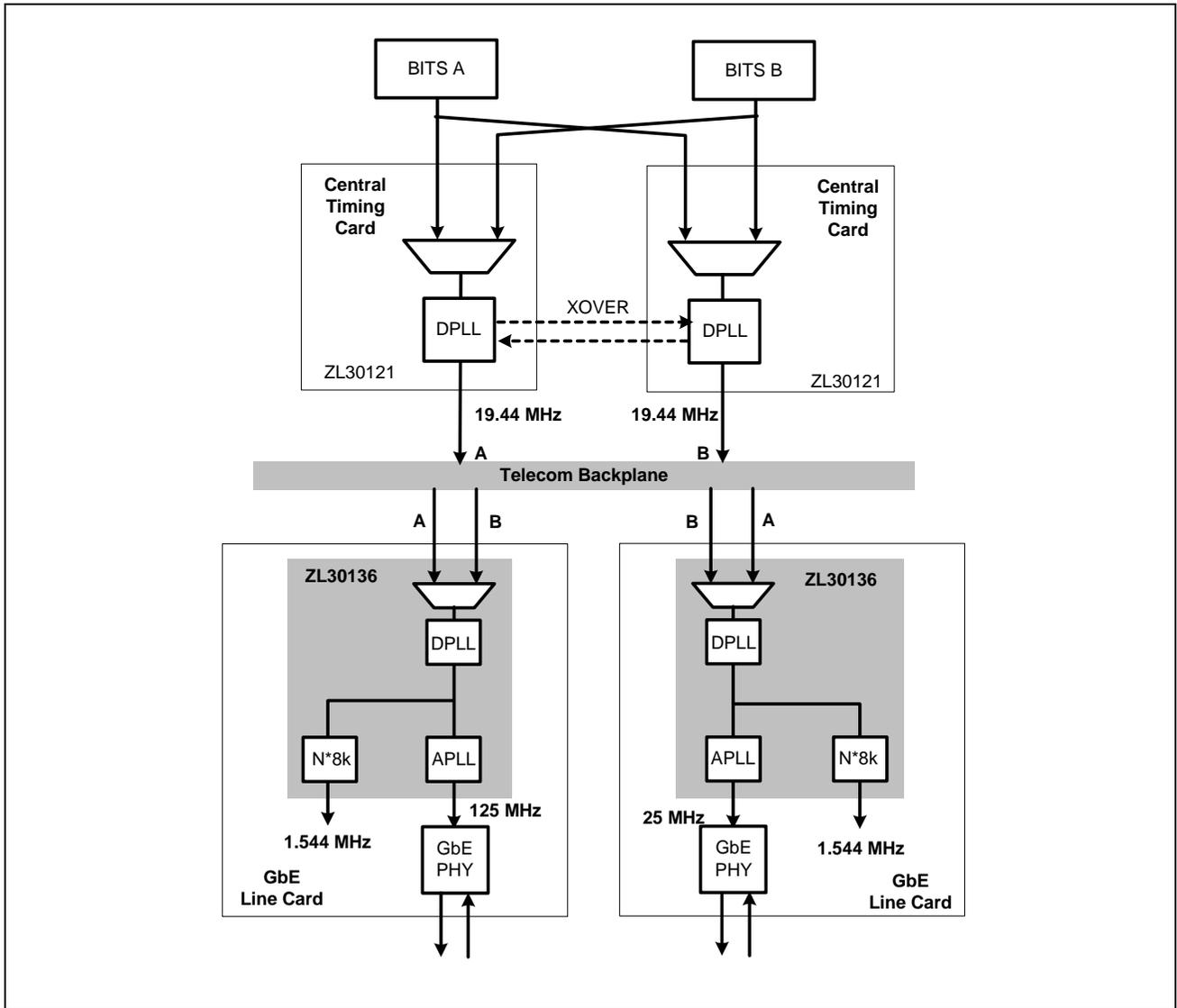
Figure 2 - Typical Application of the ZL30136
