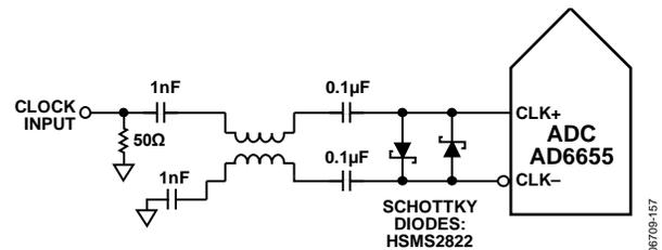
Figure 58. Balun-Coupled Differential Clock (Up to 625 MHz)
