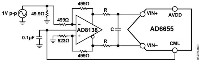
Figure 47. Differential Input Configuration Using the AD8138
