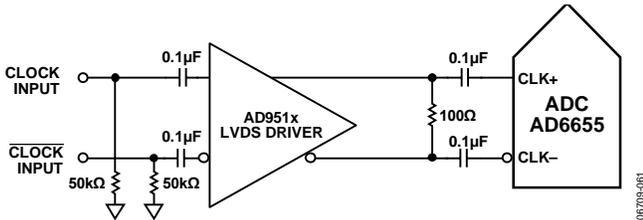
Figure 60. Differential LVDS Sample Clock (Up to 625 MHz)
