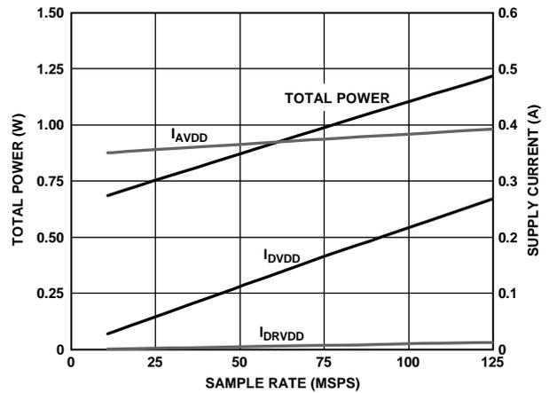
Figure 65. AD6655-125 Power and Current vs. Sample Rate
