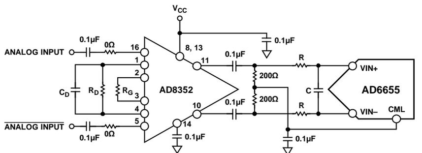
Figure 50. Differential Input Configuration Using the AD8352
