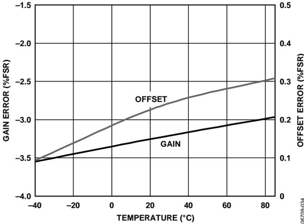
Figure 35. AD6655-150 Gain and Offset vs. Temperature
