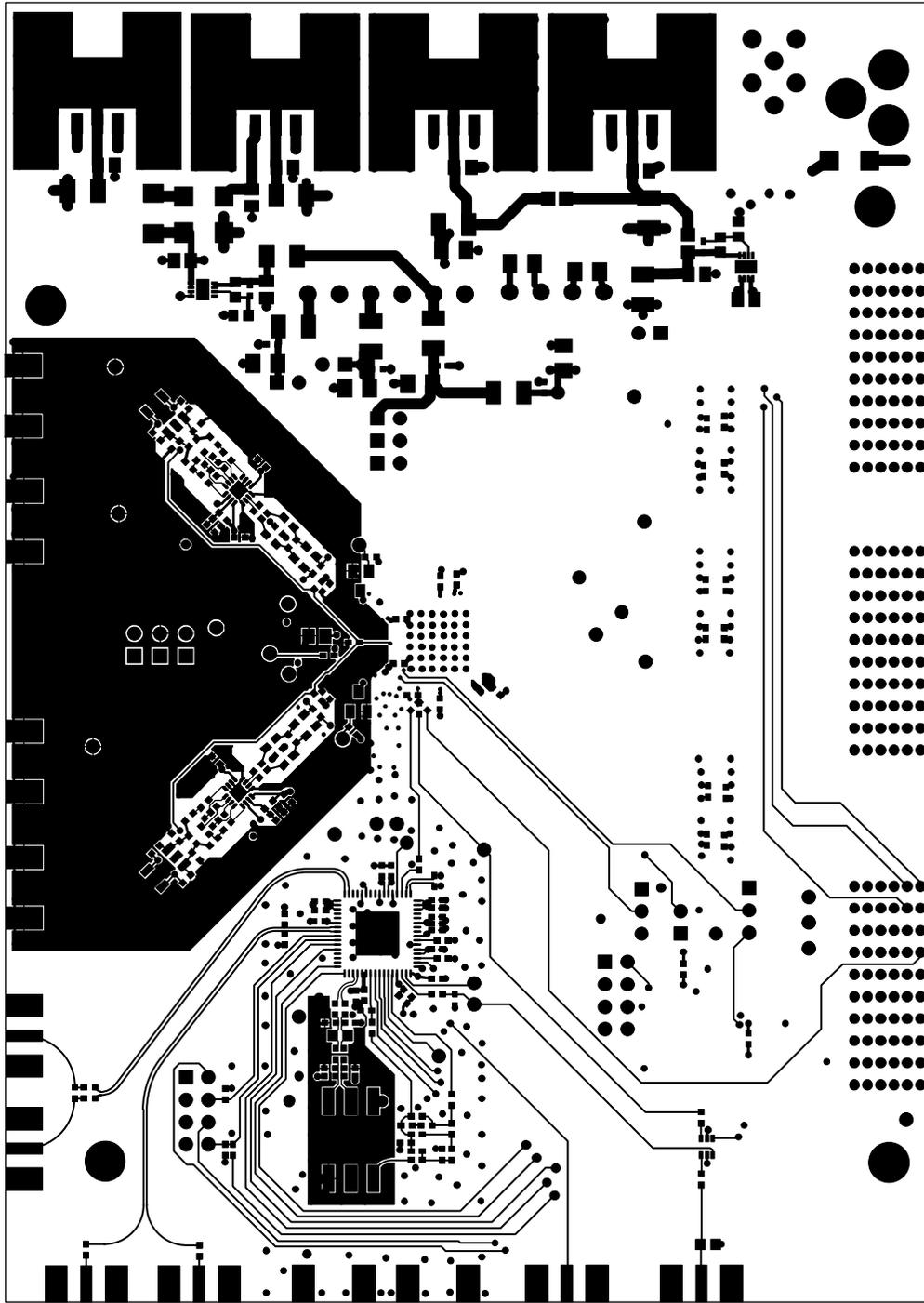
Figure 100. Evaluation Board Layout, Secondary Side (Mirrored Image)
