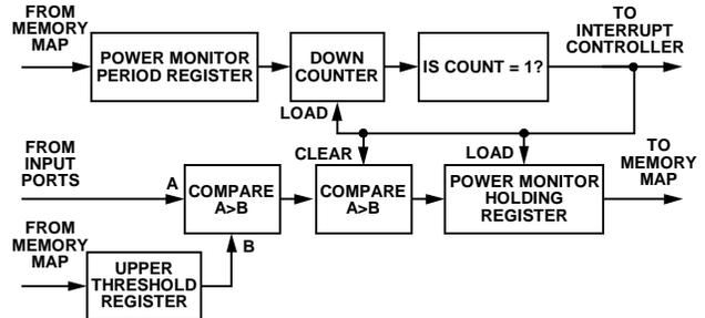
Figure 78. ADC Input Threshold Crossing Block Diagram
