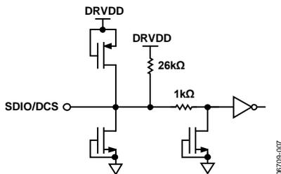
Figure 14. Equivalent SDIO/DCS Circuit or SMI SDFS Circuit
