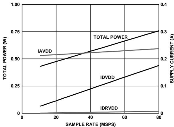
Figure 67. AD6655-80 Power and Current vs. Sample Rate
