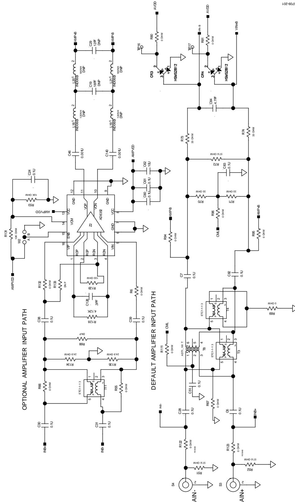
Figure 86. Evaluation Board Schematic, Channel B Analog Inputs
