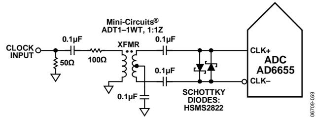
Figure 57. Transformer Coupled Differential Clock (Up to 200 MHz)
