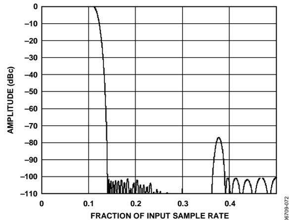
Figure 74. Half-Band Filter and FIR Filter Composite Response
