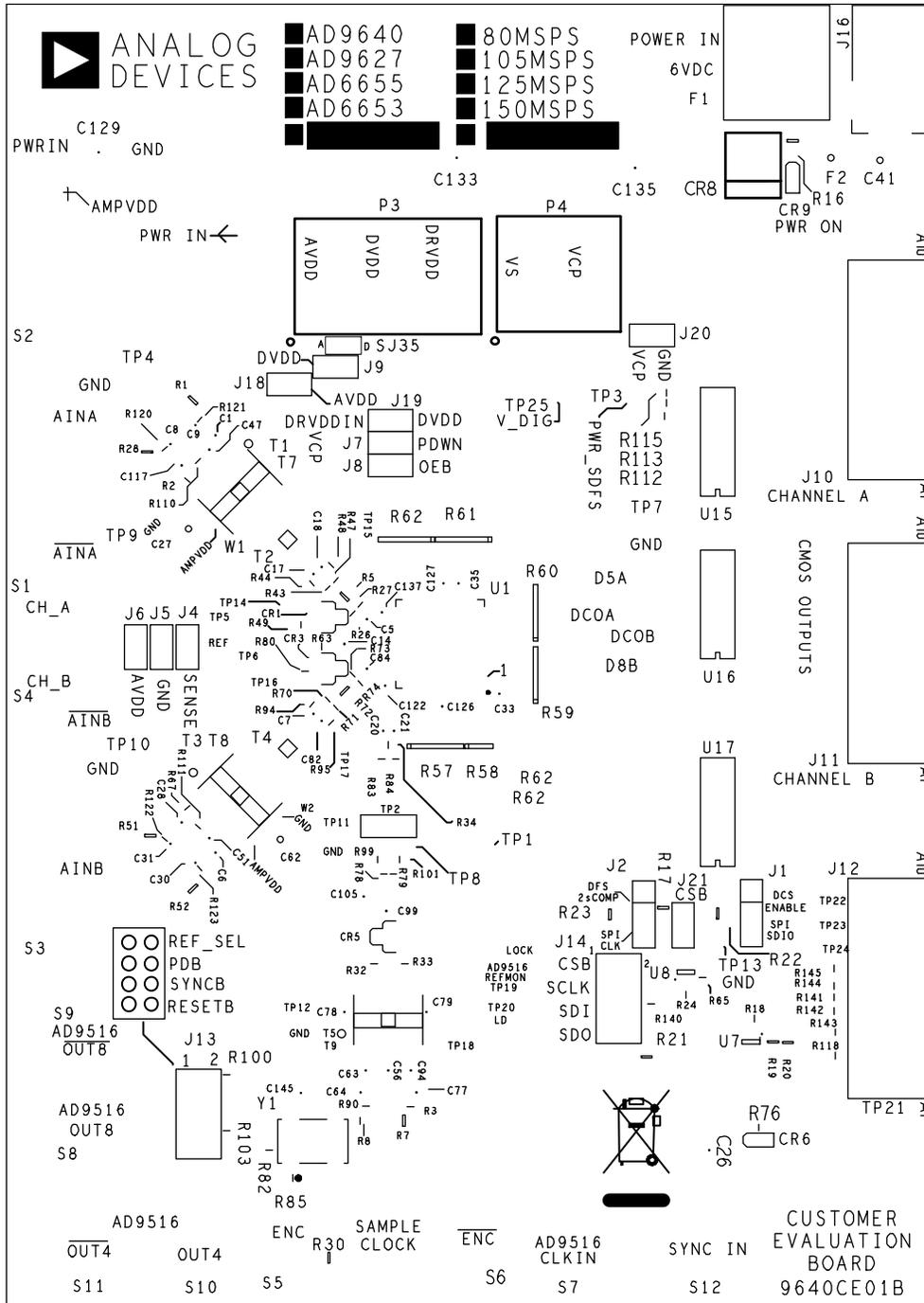
Figure 101. Evaluation Board Layout, Silkscreen, Primary Side
