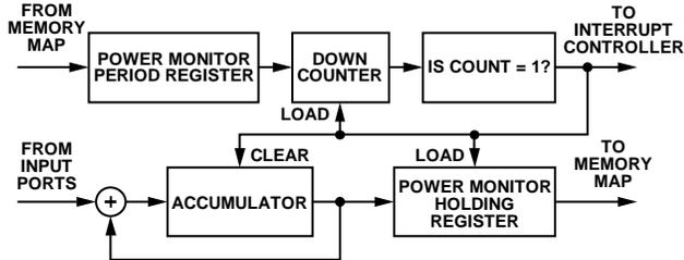
Figure 77. ADC Input RMS Magnitude Monitoring Block Diagram
