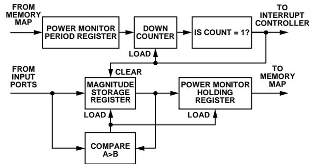
Figure 76. ADC Input Peak Detector Block Diagram
