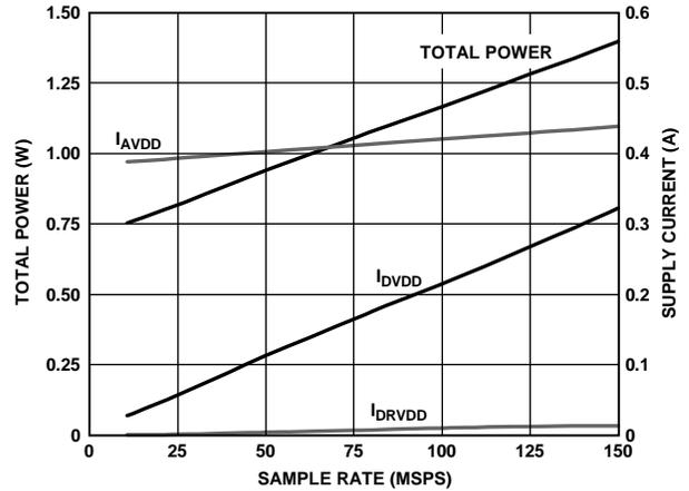
Figure 64. AD6655-150 Power and Current vs. Sample Rate
