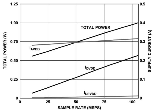
Figure 66. AD6655-105 Power and Current vs. Sample Rate
