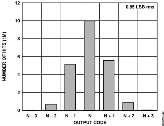
Figure 43. AD6655 Grounded Input Histogram
