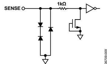
Figure 16. Equivalent SENSE Circuit
