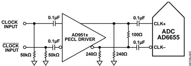
Figure 59. Differential PECL Sample Clock (Up to 625 MHz)
