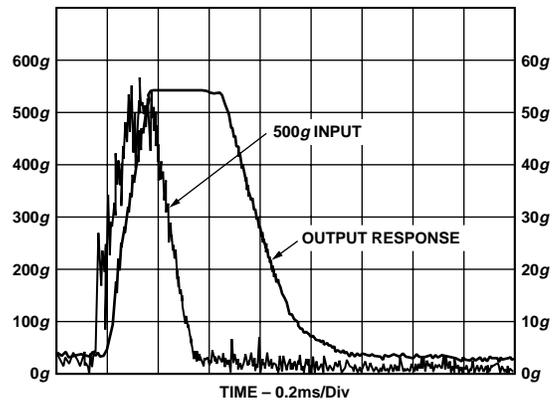
Figure 8. Typical 500 g Step Recovery at the Output
