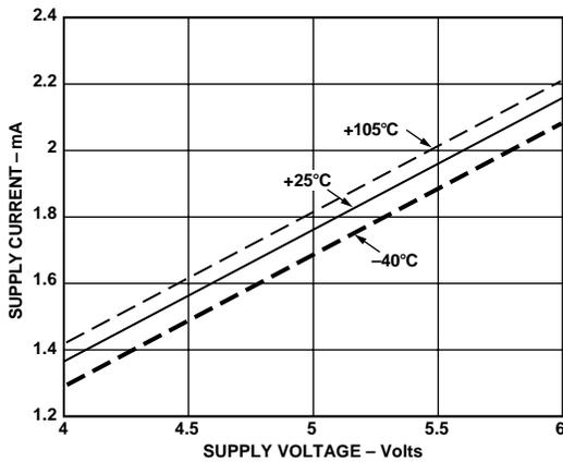
Figure 5. Typical Supply Current vs. Supply Voltage
