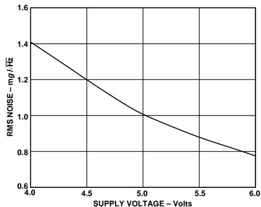
Figure 12. Noise vs. Supply Voltage
