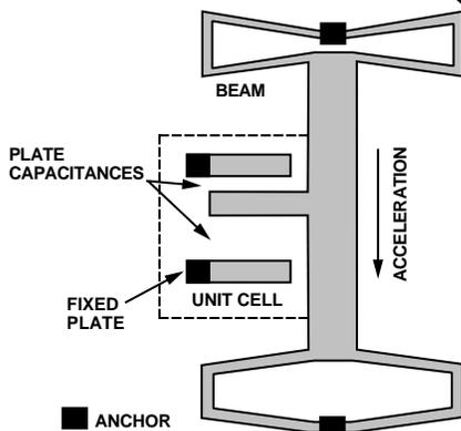
Figure 14. Simplified View of Sensor Under Acceleration
