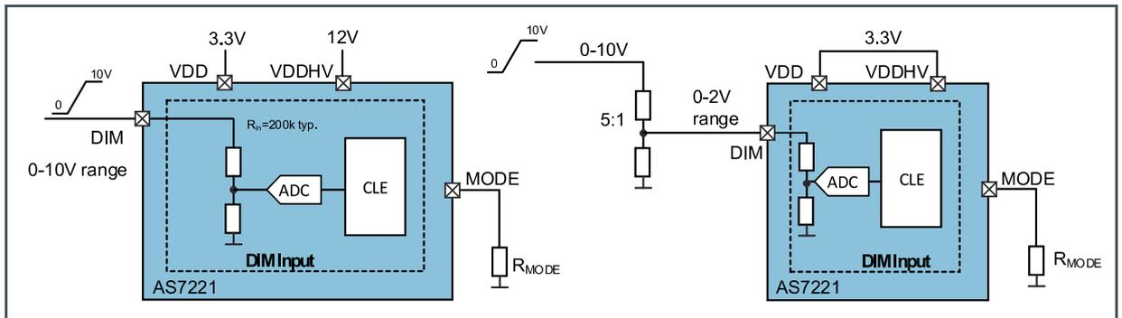
For the AS7221, dimming can be accomplished from either the input pin (DIM) or smart lighting command via the UART. For network commanded dimming, using the AS7221 Smart Lighting Command Set, the UART interface is used. To prevent flicker effects the low end of the dimming range can be adjusted via the ATDMLTL command to the provided range of the external dimming device.
