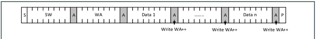
The transmission begins with the START condition, which is generated by the master when the bus is in IDLE state (the bus is free). The device-write address is followed by the word address. After the word address any number of data bytes can be sent to the slave. The word address is incremented internally, in order to write subsequent data bytes on subsequent address locations.
