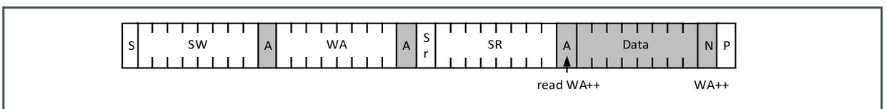
Random Read and Sequential Read are combined formats. The repeated START condition is used to change the direction after the data transfer from the master.
