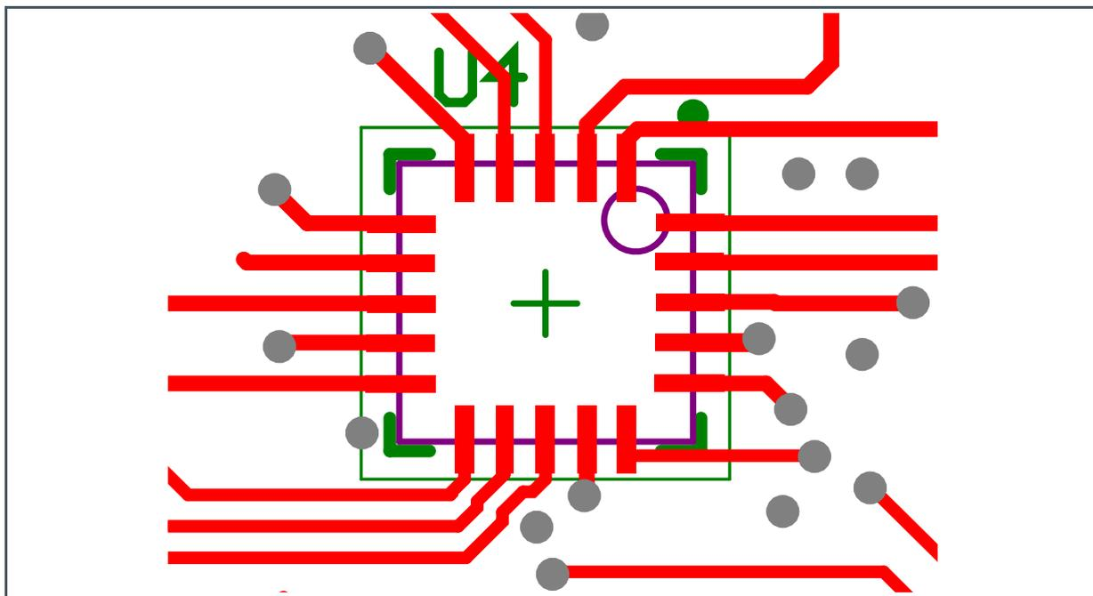
In order to prevent interference, avoid trace routing feedthroughs with exposure directly under the AS7221. An example routing is illustrated in the diagram.
