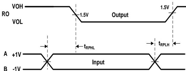
Fig.9 Receiver Propagation Delays
