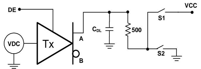
Fig.4 Transmitter enable/disable timing test load
