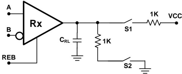
Fig.3 Receiver enable/disable timing test load
