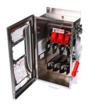
Siemens Low Voltage Circuit Protection Heavy Duty Safety Switches. Type: ENCLOSED, SAFETY SWITCH Std: CSA V. Rating: 600V A. Rating: 100A Wattage: 3W No. Of Poles: 3P F. Rating: 60Hz Action: SINGLE THROW Material: SS Enclosure: TYPE 4X. 2-3 point mounting holes. Insulation: YES O. Cycles: 10000 O. Temperature: (-20F-120F) AMBIENT TEMPERATURE Environmental Conditions: INDUSTRIAL CORROSIVE RESISTANCE
