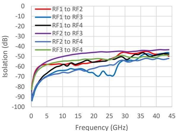
**Isolation between RF1 to RF4, RFC to RF2 On<sup>11</sup>**
