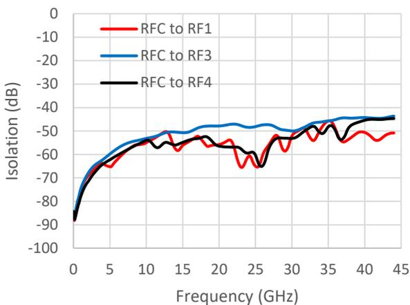
**RFC to RF1 / RF2 / RF4 Isolation, RFC to RF3 On<sup>11</sup>**
