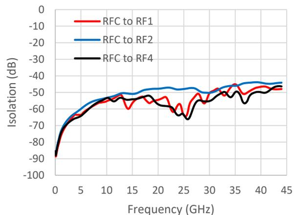
**Isolation between RF1 to RF4, RFC to RF1 On<sup>11</sup>**
