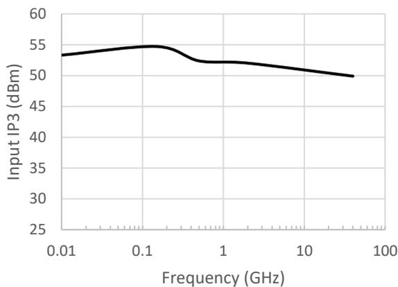
13. Input IP3 were measured using connectorized evaluation board with impedance matching. The RF input power was 14 dBm per tone with spacing of 1 MHz.
