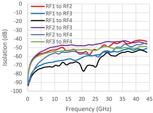
**Isolation between RF1 to RF4, RFC to RF3 On<sup>11</sup>**
