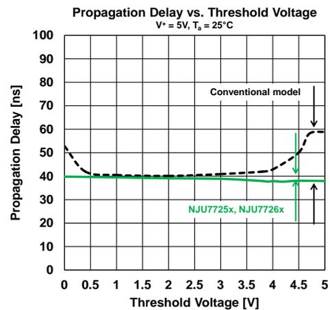
Figure 3. Propagation delay vs. Threshold Voltage
