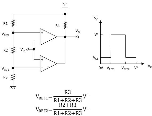
Figure 9. Window Comparator with NJU7726x
