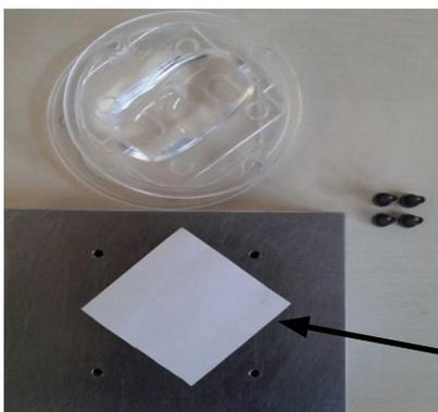
As shown in the photo, the test paper sheet is completely dry after disassembling the system.
