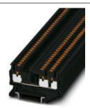
Feed-through terminal block, Connection method: Push-in connection, Cross section: 0.14 mm² - 4 mm², AWG: 26 - 12, Width: 5.2 mm, Color: black, Mounting type: NS 35/7,5, NS 35/15
