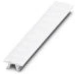
Marker for terminal blocks, Strip, white, labeled, can be labeled with: Plotter, Printed horizontally: U, V, W, N, GND, U, V, W, N, GND, Mounting type: Snap into tall marker groove, for terminal block width: 6.2 mm, Lettering field: 6.15 x 10.5 mm
