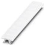
Zack marker strip, Strip, white, labeled, can be labeled with: Plotter, Printed vertically: Consecutive numbers 1 - 10, 11 - 20, etc. up to 491 - 500, Mounting type: Snap into tall marker groove, for terminal block width: 6.2 mm, Lettering field: 6.15 x 10.5 mm
