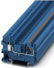
Feed-through terminal block, Connection type: Push-in connection, Screw connection, Cross section: 0.2 mm<sup>2</sup> - 6 mm<sup>2</sup>, AWG :24- 12, Width: 6.2 mm, Color: blue, Mounting: NS 35/7,5, NS 35/15
