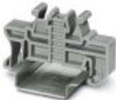
Quick mounting end clamp for NS 35/7,5 DIN rail or NS 35/15 DIN rail, with marking option, width: 9.5 mm, color: gray
