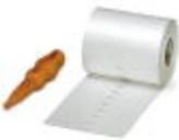
Marker for terminal blocks. Roll, white, unlabeled, can be labeled with: THERMOMARK ROLL, THERMOMARK ROLL X1, THERMOMARK X, THERMOMARK S1.1, Perforated, Mounting type: Snap into universal marker groove, Snap into flat marker groove, for terminal block width: 6.2 mm, Lettering field: 6.35 x 6.15 mm
